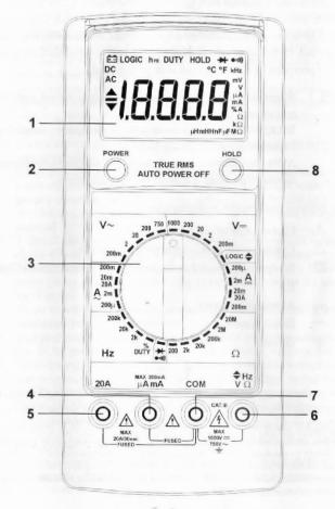
Display. 4-1/2 digit display (19999 maximum) with automatic decimal point, polarity indication. high-low logic indicators, and low battery indicator. Indicates measured value, unit of measurement, and whether dc or ac is selected (for current and voltage readings). Overrange is indicated by displaying OL.
